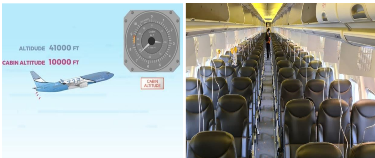
Figures 2 & 3: An illustration of a B737 aircraft animation snap shot showing the illuminated “Cabin Altitude” warning and the Cabin Altitude at 10000 feet (left); and a picture of ZS-SJF aircraft showing the deployed oxygen masks (right).
